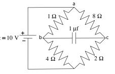
We know the electrical potential of Point "a" is 10 volts (it's connected to the high side of the battery). If we can determine the voltage drop across the 1 ohm resistor, we can determine the electrical potential at Point "b" (it'll be
